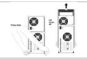
Removing the cover of the PowerCC PowerWave tower
